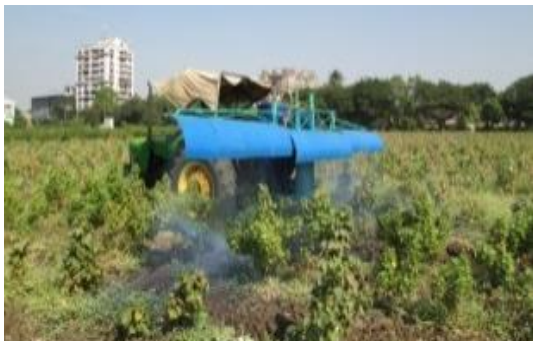
Drift control shield For Boom Sprayer
