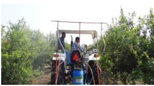
Ultrasonic Sensor Based Pomegranate sprayer
