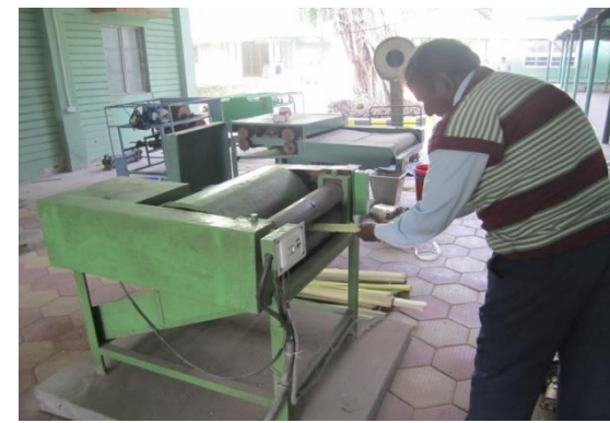
Banana fibre Extractor for textile use
