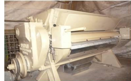
Doffing system for double roller gin to reduce dust emission
