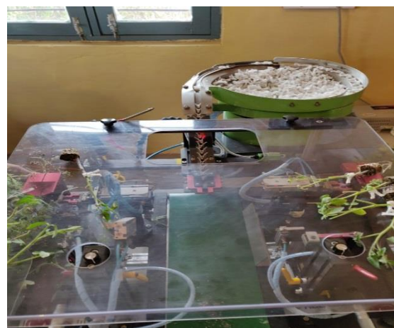
Demo of semi-automatic grafting by use of robot
